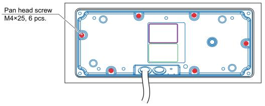
Rear side of the control unit (cover removed)
