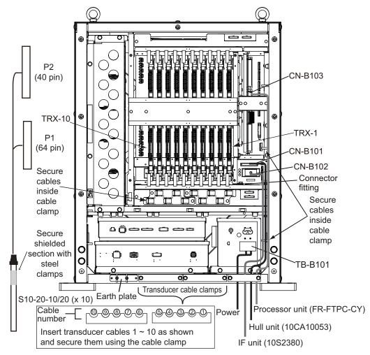
The transceiver unit is supplied with an earth plate (50 mm width, 1.5 m length) in the installation materials. Use the two wing nuts to secure the plate and connect the transceiver ground plate to the ship's earth.
