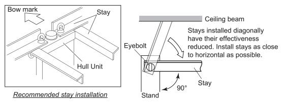
Where horizontal installation of the stays is not possible, install the stays in a diagonal manner to reduce vibration in the hull unit. Install the upper stays (attached to the top of the hull unit) in opposing directions (one facing fore, one facing aft), then attach the stays to ceiling beams. This reduces axial movement. The side stays should be installed and attached to the hull framework.
