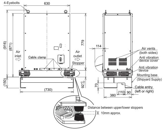
3. Fix the transceiver unit to the anti-vibration devices with M12x50 hex bolts, spring washers, plain washers and 2 x nuts (supplied). Insert the bolts from the bottom of the fixing plate.
