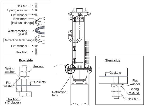
Fastening torque for all flange hex nuts: 230 N·m
