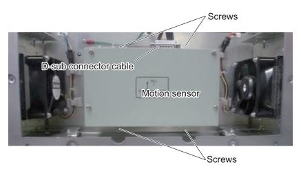
4. Connect the cable with the D-sub connector to the motion sensor socket, then secure the cable with the two screws.
