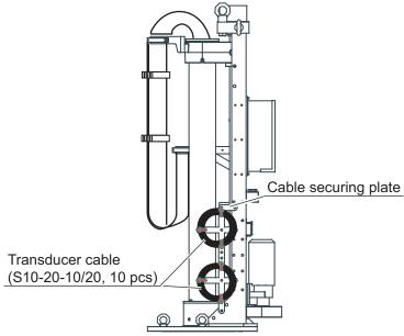
When the transducer is removed from the hull unit while installing the hull unit, reattach the transducer and route the transducer cables as shown in the following figure.
