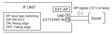
Make the connections shown below to output KP for external sonars and current indicators. This sonar transmits a keying pulse (KP) to connected external sensors when this sonar is connected and running.
