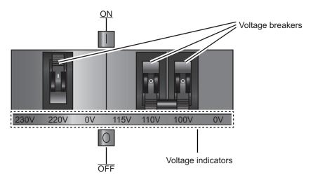
For 100/110/115V input set the double breaker on the right to ON. For 220/230V input, set the single breaker on the left to ON.
