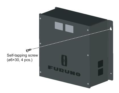
**Note:** Do not install the processor with the connectors facing upwards. Refer to the figure shown below for recommended installation.
